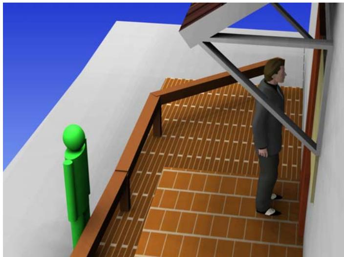
This model can predict the view from a 12mm lens + camera in the top right corner. Field of view, %Rotakin, etc. are clear even to a non-technical client, unlike relying on plans & written specifications.
