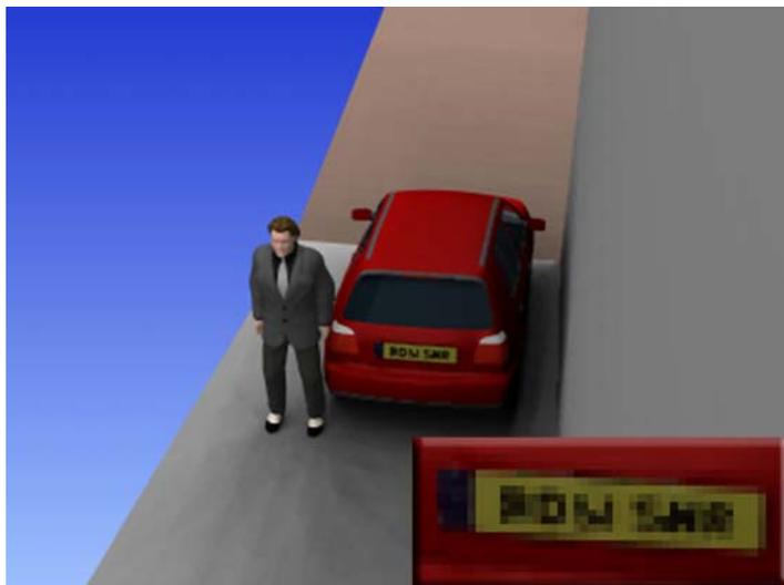
A supplier claims that their proposal will identify vehicles. With this lens and a 288x384 pixel image simulating DVR or VHS playback, the number plate is magnified (inset) and, clearly, is unsatisfactory.
